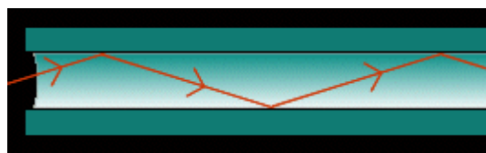
Cross section of an optical fiber.
